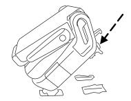
2. Install seat onto rear pin of front tub at a  $30\ \text{to}\ 45\ \text{degree}$  angle.
